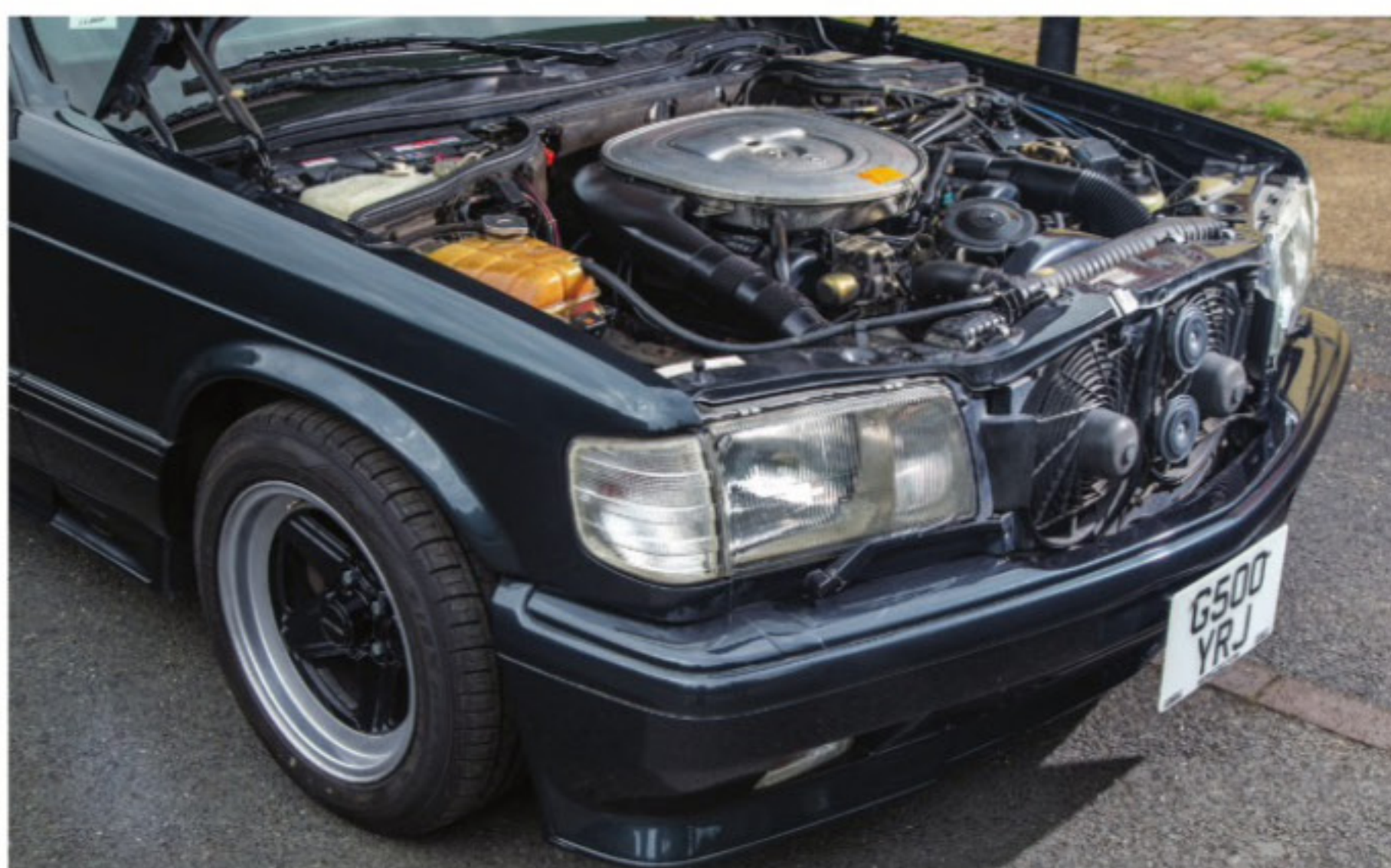
△ M117 V8 offered in six-litre form by AMG, this engine powering the illustrious Hammer models of the 1980s.
