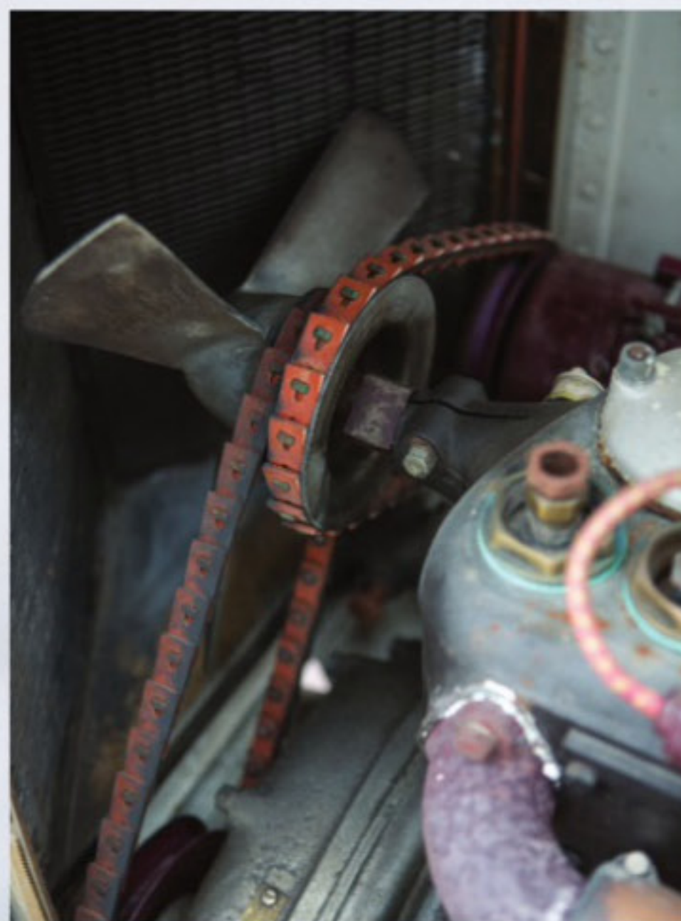
△ Intricate belt design for the four-stroke's heavy cooling fan.
